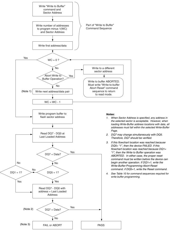
Figure 4. Write Buffer Programming Operation
