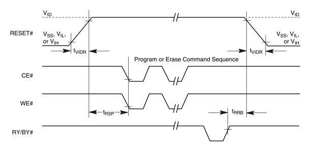
Figure 23. Temporary Sector Group Unprotect Timing Diagram
