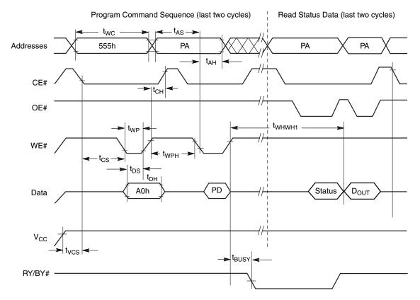
**Notes:.** PA = program address, PD = program data, D<sub>OUT</sub> is the true data at the program address.
