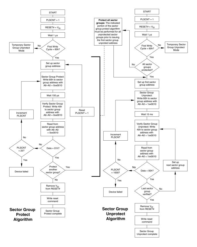
Figure 2. In-System Sector Group Protect/Unprotect Algorithms
